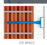
MAGNNUM FIX 3 ALMT - INSULATED DOWEL PLATE WITH METAL PIN AND PLASTIC PLATE
